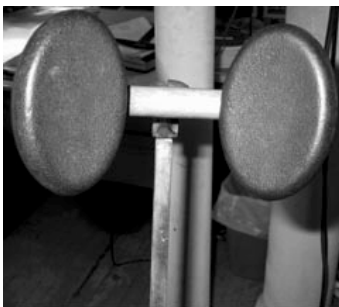
A model of the headrest structure before installation of the vibration device.
